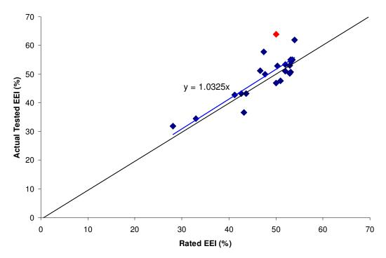
Figure 1. Rated vs. Actual Energy Efficiency Index of Refrigerators<sup>1</sup>
