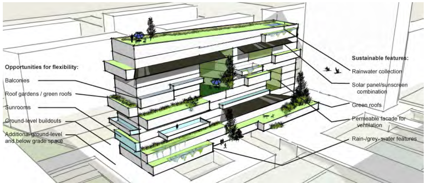
3.9. Detail of a typical building and its energy harvesting formal features
