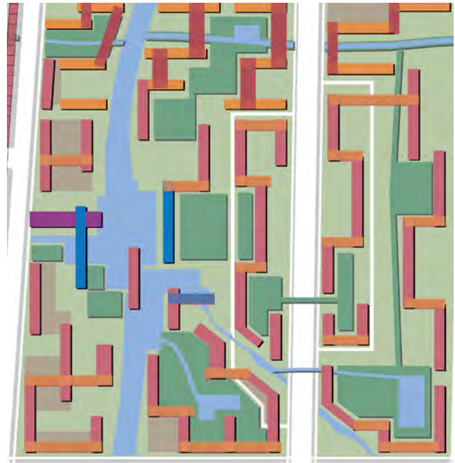
3.29 Site plan showing N-S slabs and suspended E-W links
