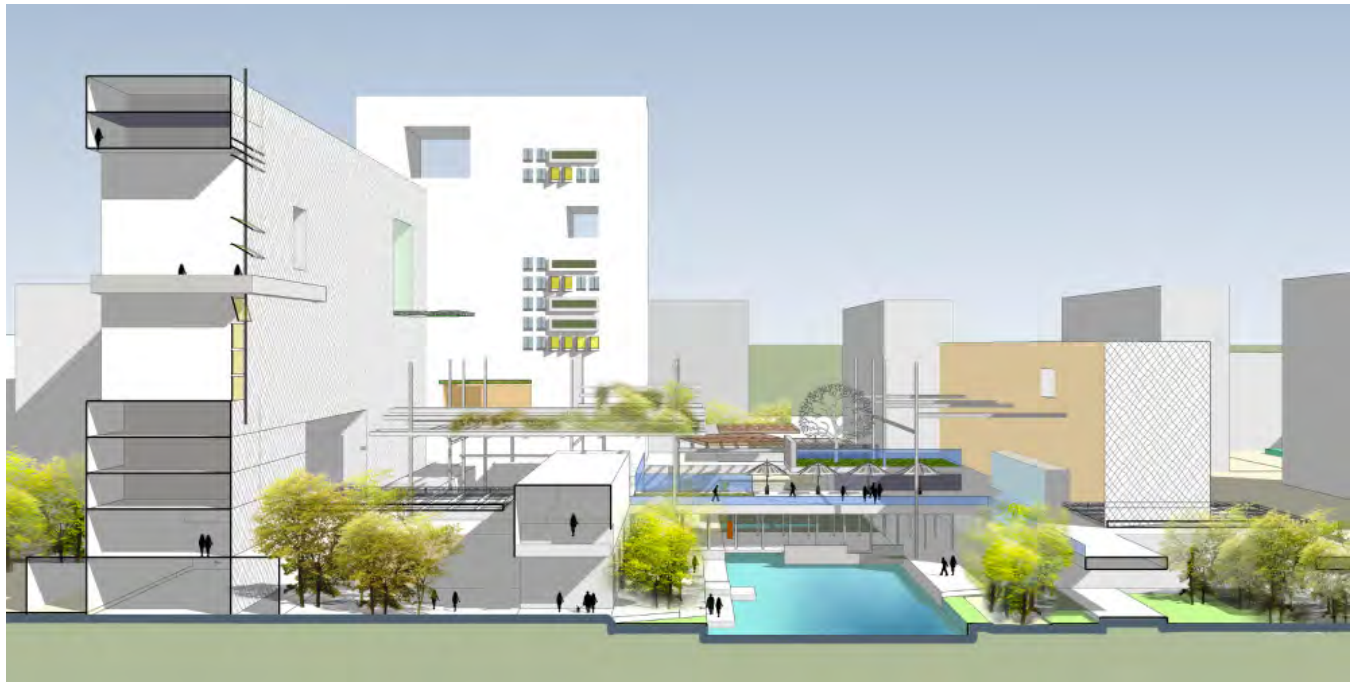
3.10. Cluster section illustrating water catchment area achieved through ground plane manipulations
